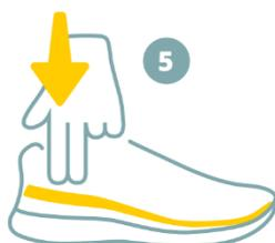
Check if the STAPPONE sensor insoles are in full contact with the shoes.
