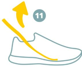
Pull on the heel area of the STAPPONE sensor insoles to remove it from your shoe.
