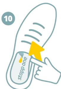
To remove the STAPPONE sensor insoles, lift sensor insole in medial mid foot area.
